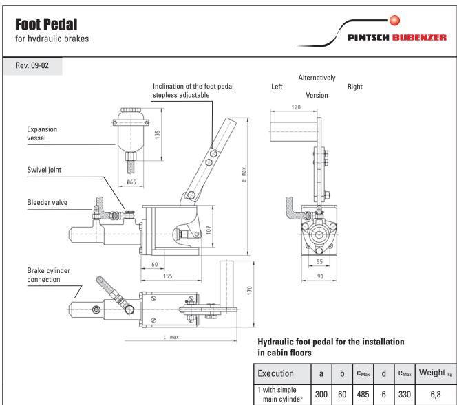
In order to operate two brakes synchronously by one foot pedal, the pipe connections from the foot pedal to each brake must be of the same length.
