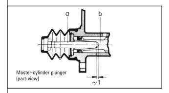
When actuated, the foot pedal is held by a pressure spring in the "off"-position against a stop, whereby there should be about 1 mm play between the plunger (a) and the top of the piston (b). This is to be taken into consideration if the factory setting of the stop has been disturbed.
